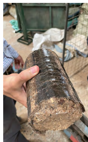
Regen Organics' (previously Sanergy) faecal sludge and agriwaste treatment plant in Ngelani City, Kenya (left and center). Faecal sludge treatment process output product (briquette) in Sanivation's Naivasha (Kenya) FSTP (right). ©Anton Jantunen/SHF
